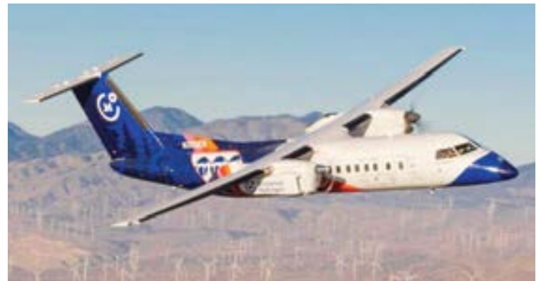
UH Lightning McClean : Photo Credit: Universal Hydrogen Photo Caption: "Lightning McClean," Universal Hydrogen's zero-emission Dash 8-300, cruising the skies of Mojave.
